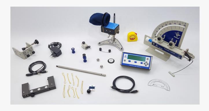
Set of projectile launchers, trimmer, with 12-function digital multitimer, sensors
